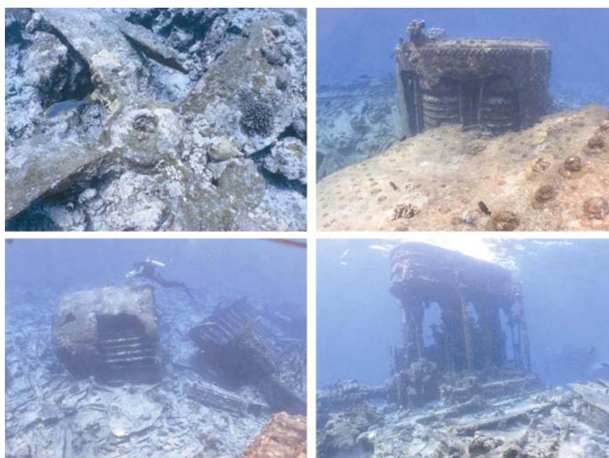
Figure 3. Remains of propeller, boilers and flywheel of the shipwreck off Minicoy Island.
