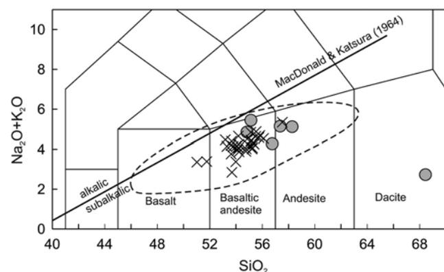
**Figure 5.** Total alkalis versus silica (wt %) for glass matrices of lithic fragments from AL-5 (grey circle) and AL-6 (cross). The fields are from Le Maitre<sup>19</sup>, and the boundary between sub-alkalic and alkalic compositions is from Macdonald and Katsura<sup>20</sup>. Relevant compositional fields are marked. The dashed envelope represents the known composition of Barren Island lavas<sup>8,9,17,21</sup>.
