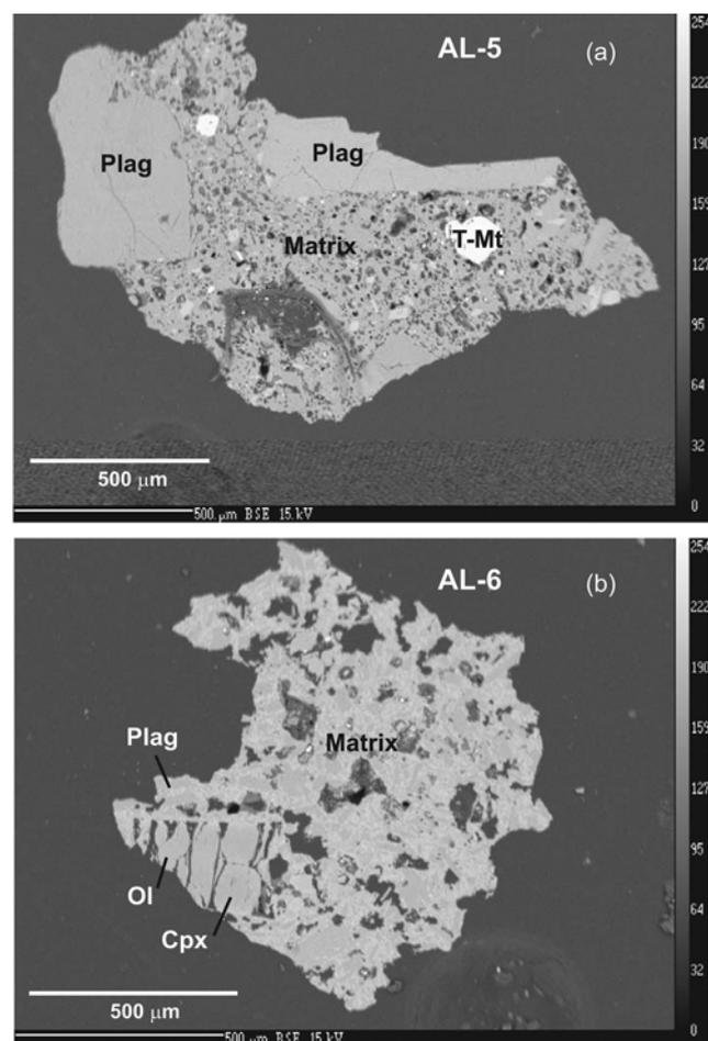
**Figure 4.** Backscattered X-ray images of typical lithic clasts from AL-5 and AL-6. Mineral grains (phenocrysts) and vesicular matrix are marked. Plag, Plagioclase; T-Mt, Titaniferous magnetite; Ol, Olivine; Cpx, Clinopyroxene.
