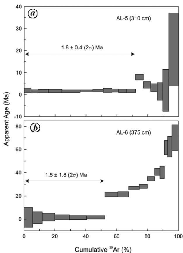
**Figure 6.** Step-heating  $^{40}\text{Ar}$ – $^{39}\text{Ar}$  apparent age spectra for plagioclase separates from (a) AL-5 and (b) AL-6. Plateau ages, which are the weighted means of contiguous, concordant step ages comprising >50% of the total gas released, are indicated. Box heights and errors on ages are at 2 $\sigma$ . Relevant data are given in Table 1.
