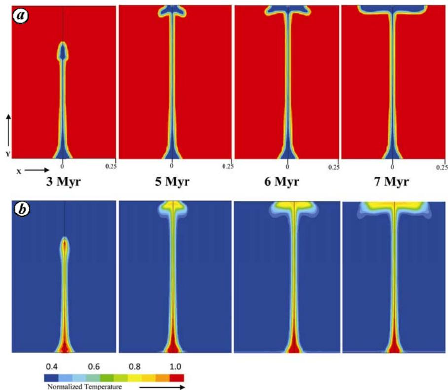
**Figure 4.** Successive stages of the plume head geometry in model simulations performed with a higher influx rate ( $Re = 18$ ). The values of  $\Delta\rho$  and  $R$  are the same as in the model shown in Figure 3. Plume shapes defined by (a) phase and (b) thermal boundaries. Scale bar shows the normalized temperatures.
