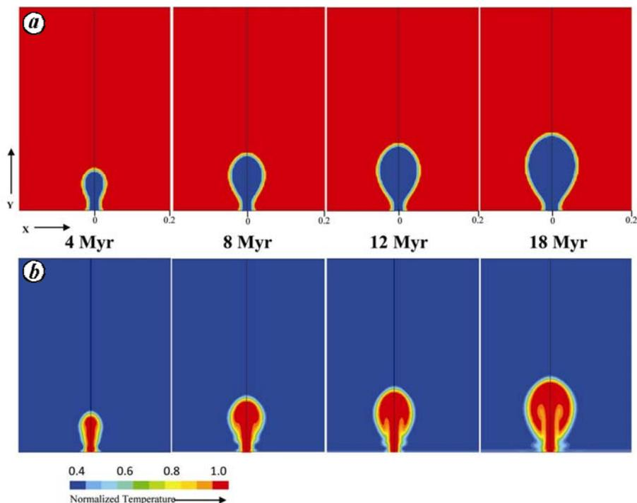
**Figure 3.** Progressive development of a plume in ballooning mode in VOF models run with high density contrast ( $\Delta\rho = 1.2$ ) and low influx rate ( $Re = 6$ ). Viscosity ratio  $R = 1$ . Mapping of the plume shapes by (a) phase and (b) thermal boundary. The temperature scale has been normalized by the initial temperature of plume material.
