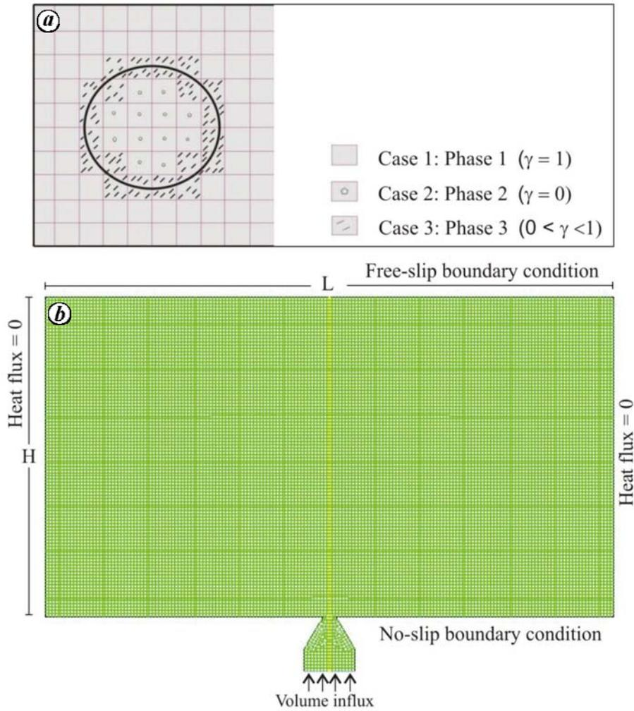
**Figure 2.** *a*, Basic mathematical concept of volume averaging in a two-phase fluid system.  $\gamma$  is a phase indicator function (see text for details). *b*, An initial volume-of-fluid (VOF) model showing the boundary conditions chosen for numerical simulation.
