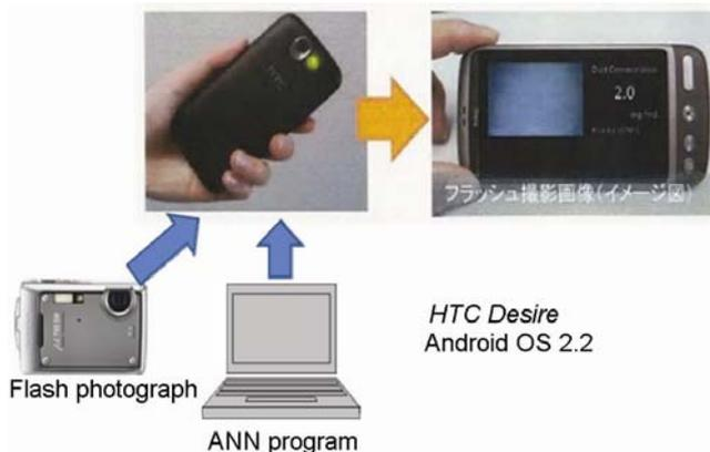
Figure 1. Dust measuring system using mobile phone camera.
