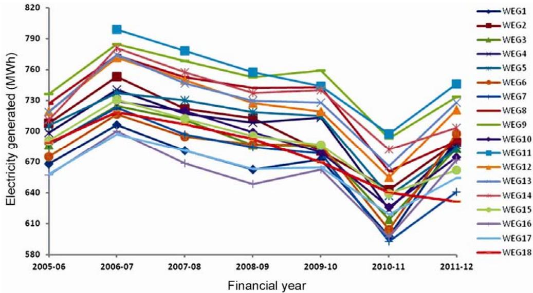
Figure 2. Graph of electricity generated by the 18 wind electric generators in each financial year from 2005 to 2011.
