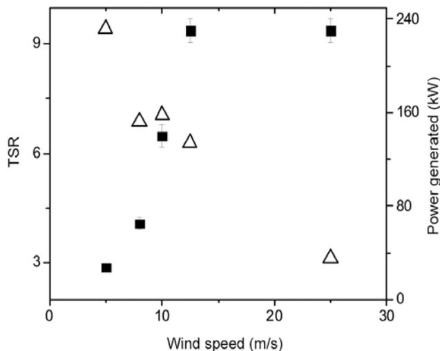
Figure 6. Variation of tip speed ratio (TSR; Δ) and power generated (■) by WEGs as a function of wind speed.
