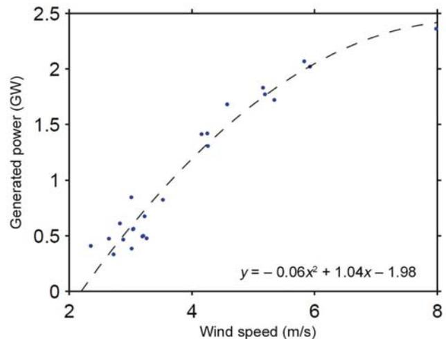
Figure 8. Variation of monthly averaged wind speed against the power generated by all the 18 WEGs in the farm. Wind speed source – YOTC data at 10 m height from May 2008 to April 2010 interpolated to latitude and longitude of 76.4°E and 14.2°N.
