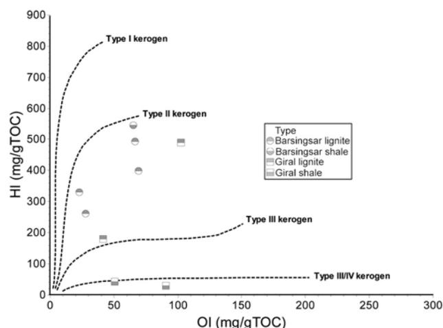
**Figure 6.** Plot of hydrogen index (HI) versus oxygen index (OI) showing organic matter type.
