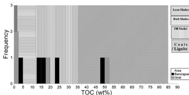
**Figure 3.** Total organic carbon content of lignite and shale.
