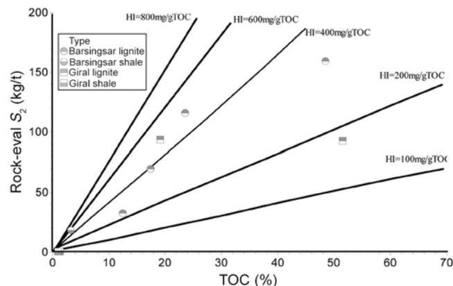
**Figure 4.** S<sub>2</sub> versus TOC plot for lignite and shale.
