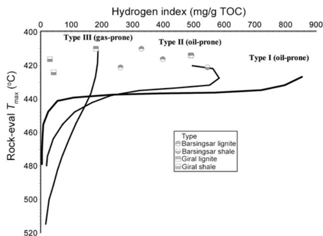
**Figure 5.** Plot of hydrogen index versus Rock-Eval  $T_{\max}$  showing organic matter type.
