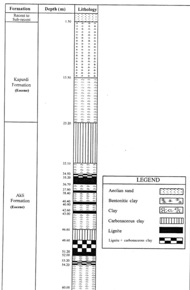
**Figure 2.** Litholog of a well from Giral area.
