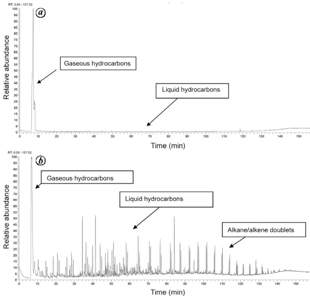
Figure 7. Pyrolysis gas chromatograms of (a) shale from Giral (Giral 2a) and (b) lignite from Barsingsar (Barsingsar 2b).
