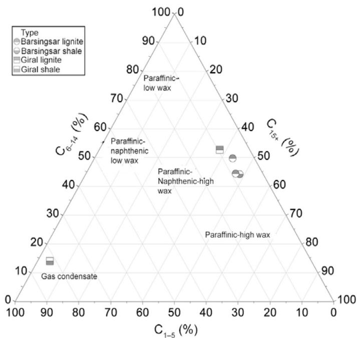
Figure 8. Oil and gas generation potential of lignite and shale based on distribution of light, medium and heavy hydrocarbons.
