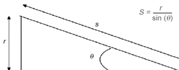
where,  $\theta$  is the slope at the point,  $r$  the sea-level rise during the 20th century and  $s$  the shifting of the coastline per unit area.
