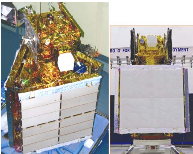
Figure 2. Stowed configuration of RISAT-1.
