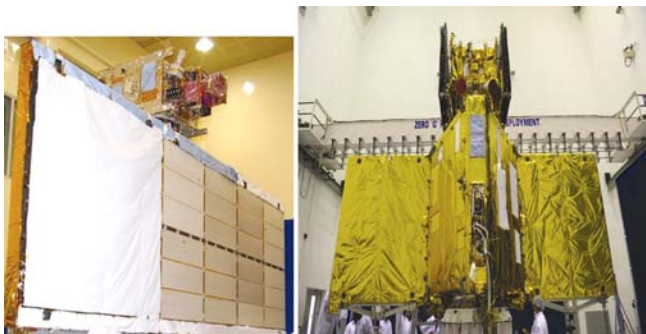
Figure 3. Deployed configuration of RISAT-1.
