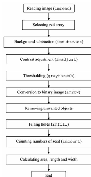
**Figure 1.** Flow diagram for measurement of dimension by image analysis.
