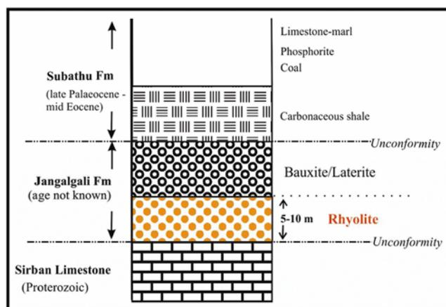
**Figure 2.** Simplified litholog of Jammu region showing the stratigraphic position of rhyolite in the unconformity zone of Jangalgali Formation.
