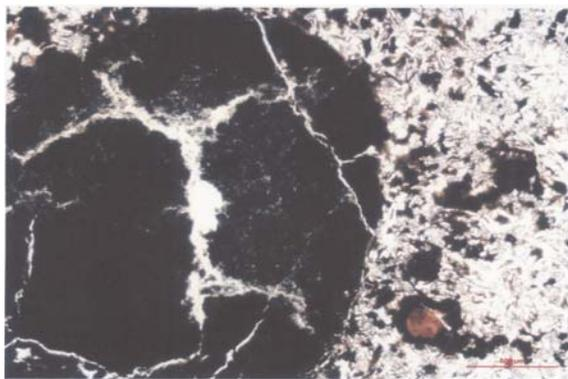
**Figure 2.** Photomicrograph of the vesicle with greyish-green nontronite exhibiting cracks (scale – 600  $\mu\text{m}$ ).
