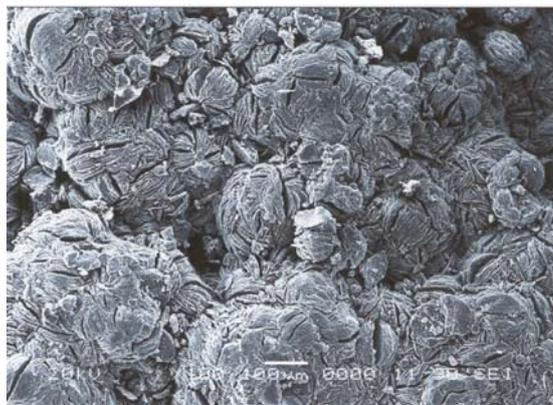
**Figure 3.** Scanning electron photomicrograph exhibiting delicate aggregates of spheroids with well-crystallized dioctahedral sheets of nontronite (scale – 50  $\mu\text{m}$ ).
