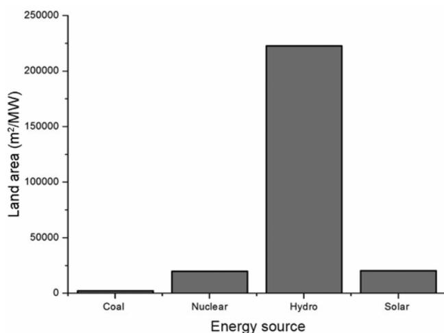
**Figure 1.** Mean values of land area required to set up a typical power plant for different energy sources.
