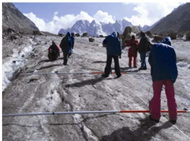
**Figure 3.** Operation of the multiple low frequency antenna on the ablation zone of Chhota Shigri glacier.
