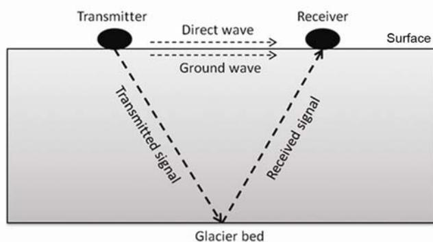
**Figure 2.** GPR set up on the ablation zone of Chhota Shigri glacier.
