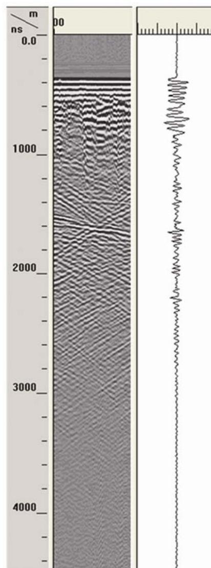
**Figure 4.** Field data collected through GPR and trace window (Line scan and Wiggle).
