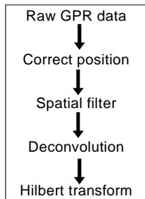
**Figure 5.** Processing step of the collected GPR data.
