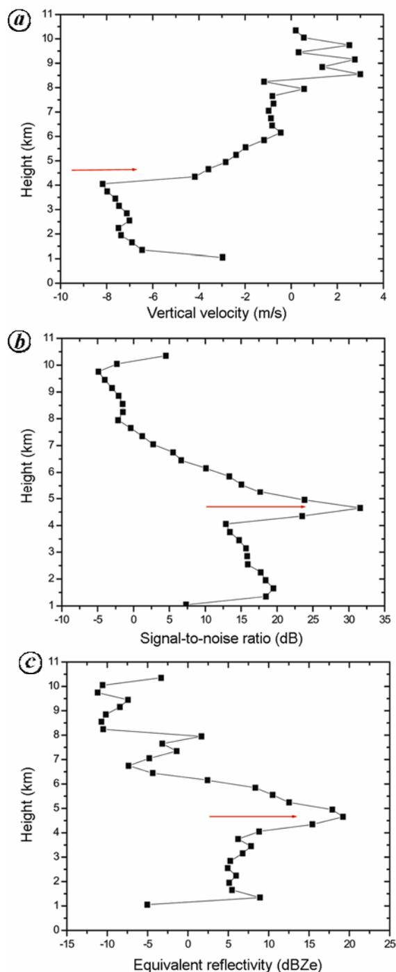
**Figure 5.** Altitude profile of (a) vertical Doppler velocity (–ve downward, met convention), (b) detectability signal-to-noise ratio and (c) equivalent reflectivity during stratiform rain, observed on 25 July 2005, 0800 h IST.
