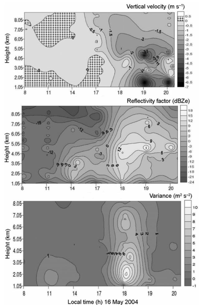
**Figure 6.** The observed parameters during convective rain are vertical velocity in  $\text{ms}^{-1}$ ; negative values indicate downward motion (top panel), reflectivity in dBZe (middle panel) and spectral width ( $\text{ms}^{-1}$ ); bottom panel).
