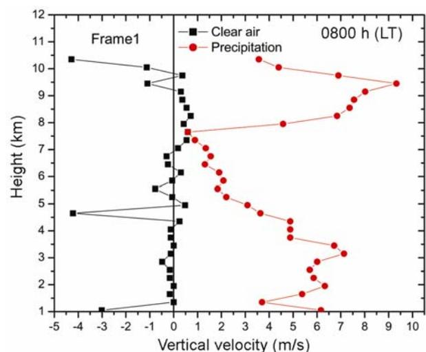
**Figure 1.** Observed typical clear air and precipitation signal measured in  $\text{ms}^{-1}$  (+ve downward, radar convention), 25 July 2005, 0800 h IST. This frame is a representative of the observation.
