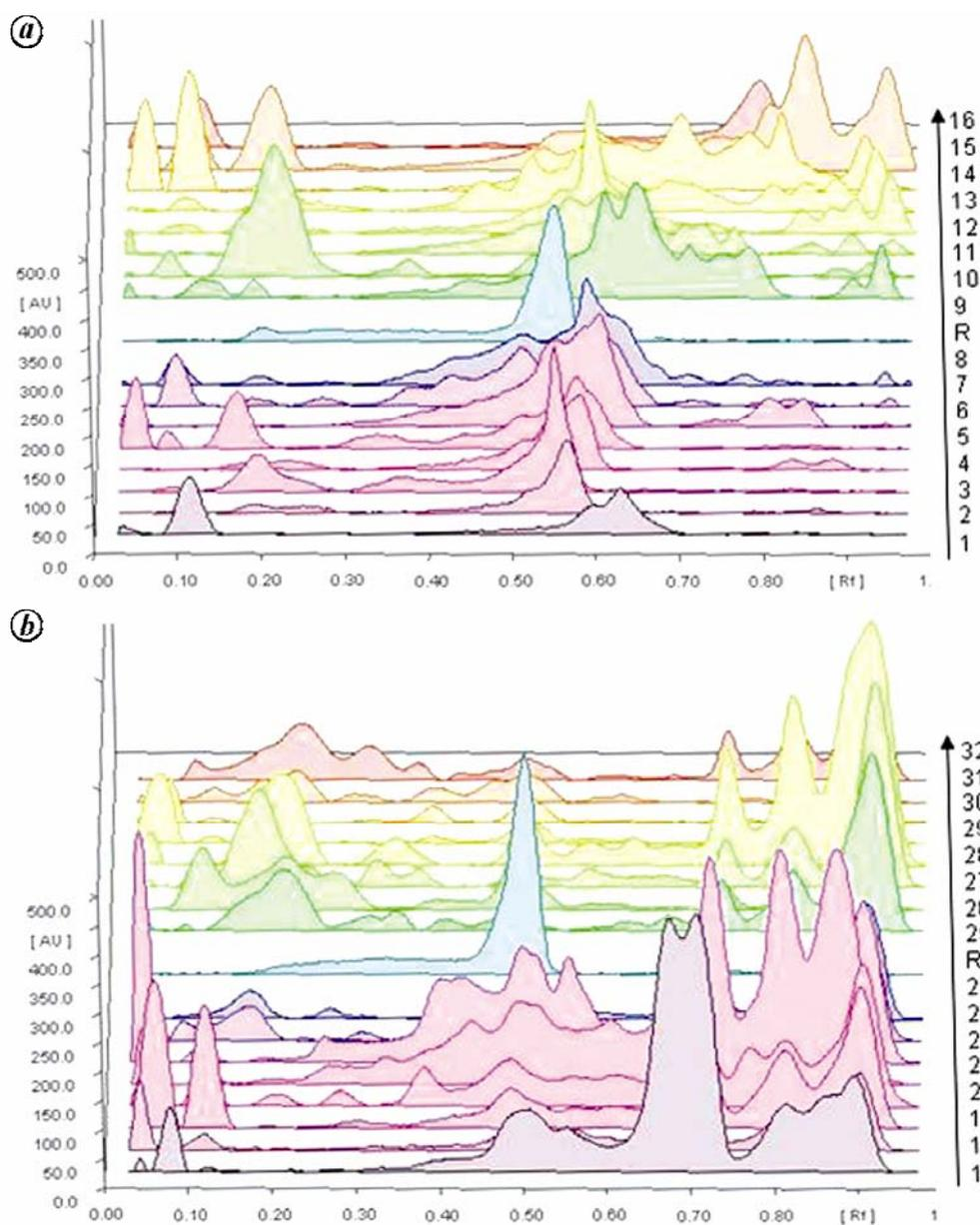
**Figure 5.** TLC densitometric scanning profile at 400 nm (samples no. 1–32; R, quercetin).
