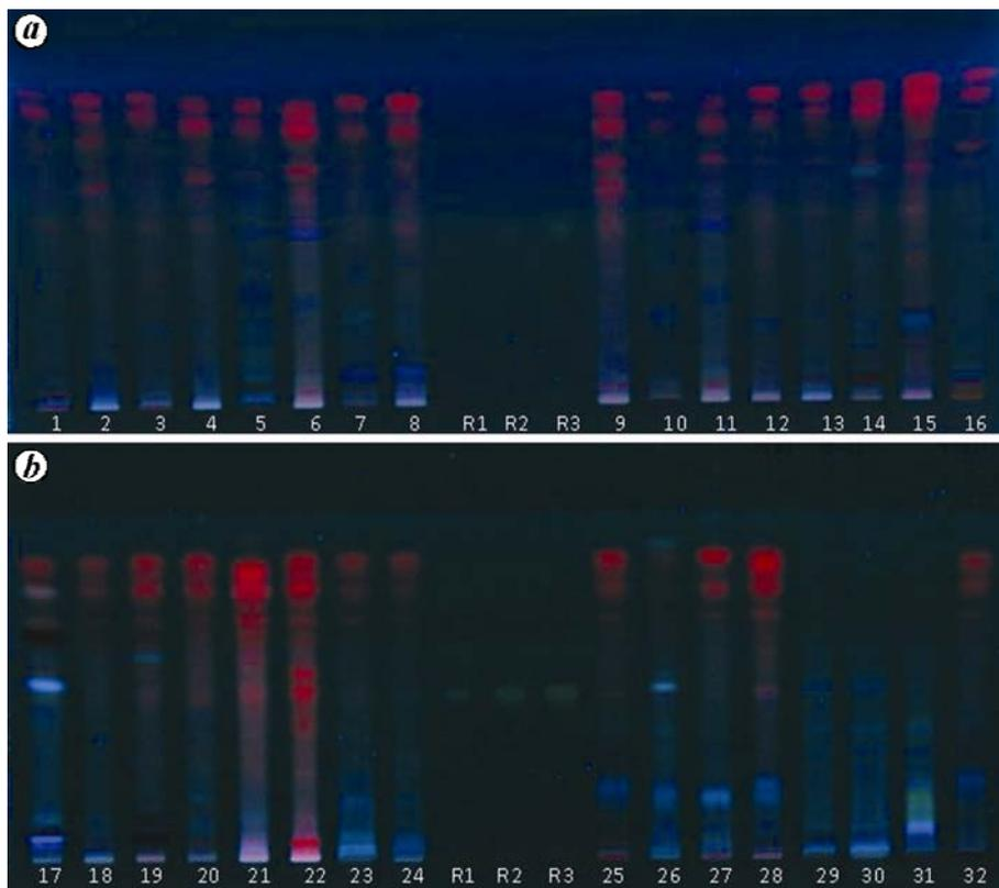
**Figure 3.** TLC showing detection of quercetin in fern samples (samples no. 1–32; R1–R3, Quercetin) under 366 nm.
