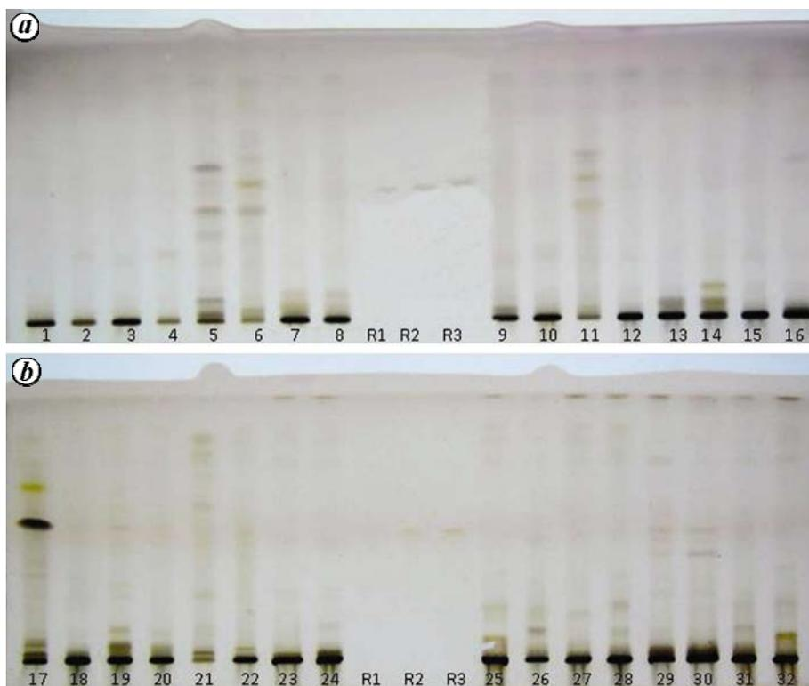
**Figure 4.** TLC showing detection of quercetin in fern samples (samples no. 1–32; R1–R3, Quercetin) under visible light after derivatization.
