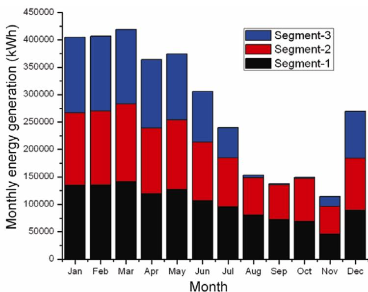
**Figure 2.** Contribution of all the three segments in the total power generation during 2010.
