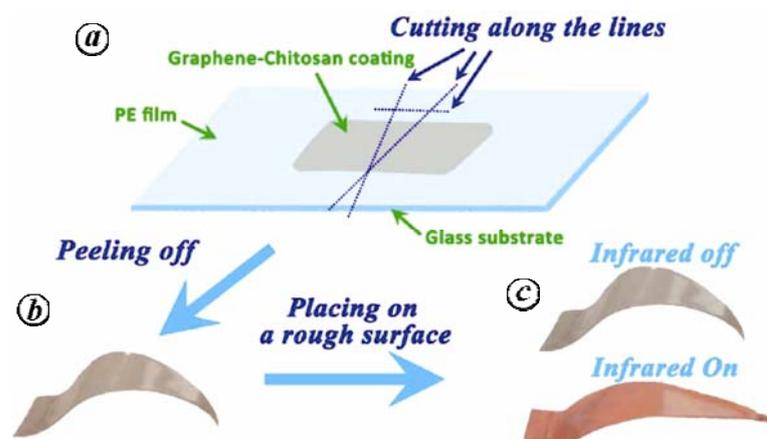
**Figure 1.** Schematic procedure for the fabrication of infrared-triggered artificial worms. **a**, Triangle-shaped area was cut out as is shown by dashed lines. **b**, The cut-out area was peeled off, after which the strip automatically transformed into a curled state. **c**, The two different states with and without IR irradiation, which shows a typical crawling mechanism like the real worms. From Wu *et al.*<sup>10</sup>. Reproduced by permission of The Royal Society of Chemistry.
