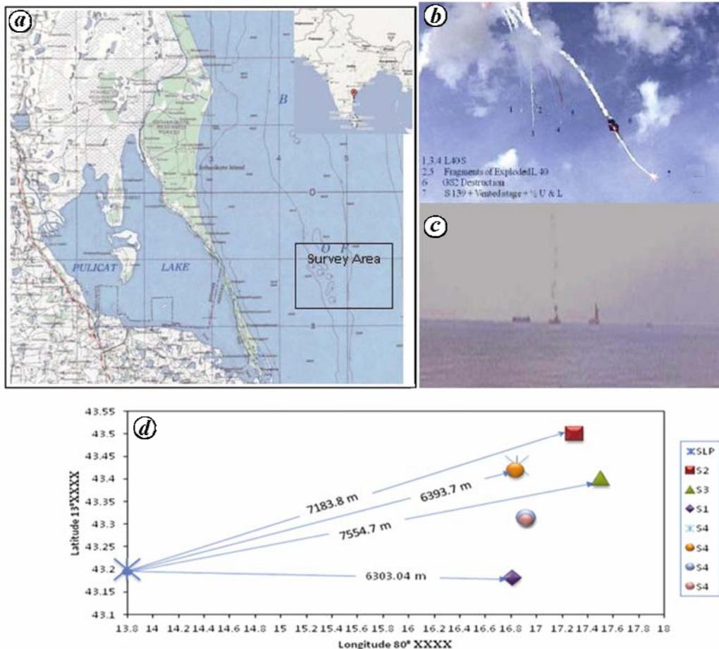
**Figure 1.** *a*, Location map. *b*, Disintegration and fall of Geosynchronous Satellite Launch Vehicle debris. *c*, L-40 impact on the sea. *d*, Relative position and distances of recovered L-40 engines from the launch pad (SLP).
