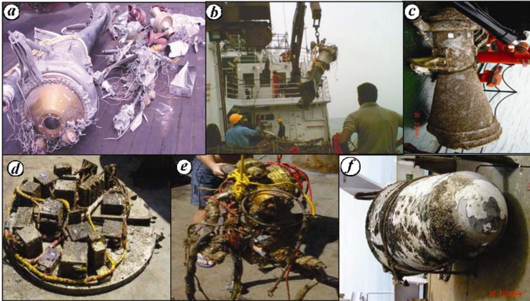
**Figure 3.** Photograph of recovered engines and their parts. *a*, S-3 engine; *b*, S-2 engine; *c*, S-1 engine; *d*, S-4 base electronics plate; *e*, S-4 engine parts and *f*, S-4 nose cone.
