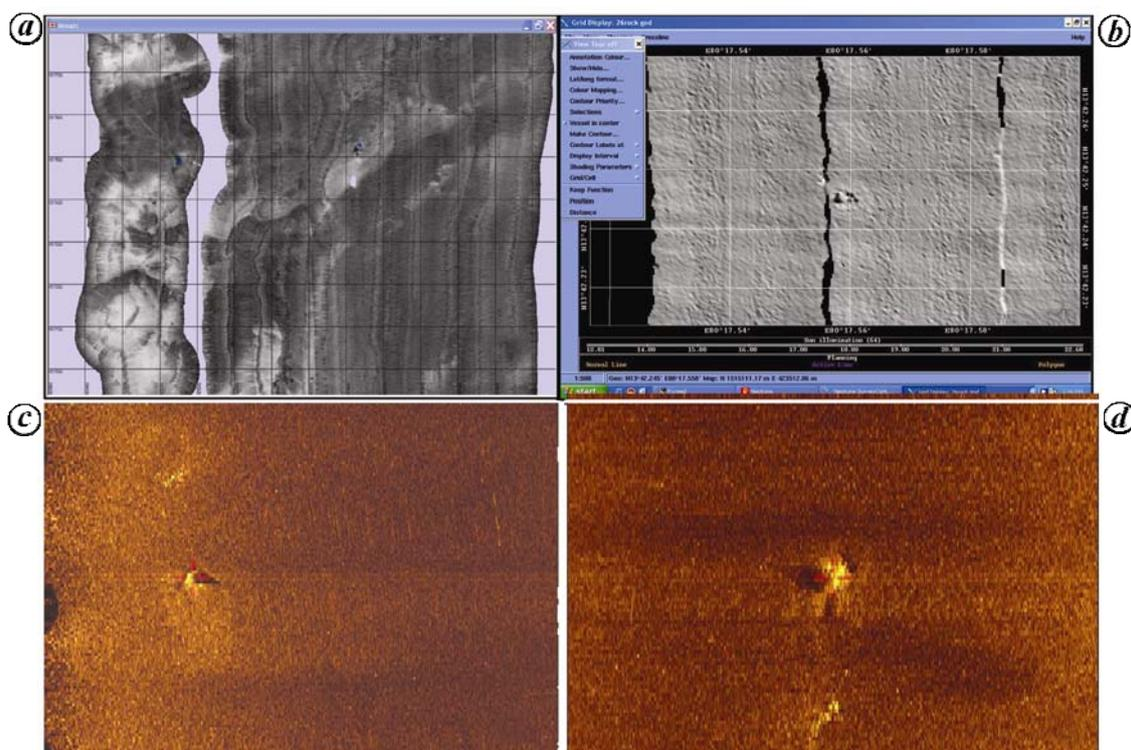
**Figure 2.** Identification of targets in bathymetric survey. *a*, Geoswath survey. *b*, EM1002 Survey. *c*, *d*, Sonar images of S-4 nose cone observed from different directions.
