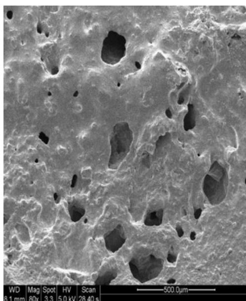
**Figure 5.** SEM image of porous CO-p(MCS) polymer scaffold.
