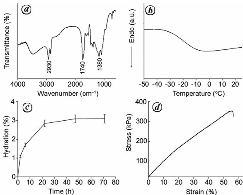
**Figure 2.** Cured CO-p(MCS) polymer characterization. *a*, FTIR spectrum; *b*, DSC thermogram; *c*, Hydration profile; *d*, Stress–strain curve.
