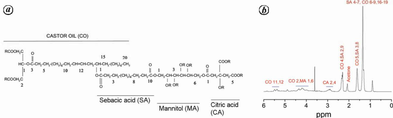
**Figure 1.** *a*, Castor oil based polyester (CO-p(MCS)) structure; *b*, <sup>1</sup>H NMR spectra of CO-p(MCS) in acetone.
