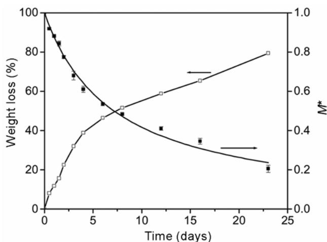
**Figure 3.** CO-p(MCS) degradation profile in PBS solution at pH 7.4 and the best fit for degradation using normalized weight ( $M^*$ ).
