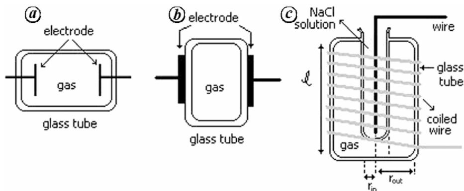
Figure 1. *a*, Metal electrode; *b*, Electrode-less planar and *c*, An ozonizer as discharge systems.
