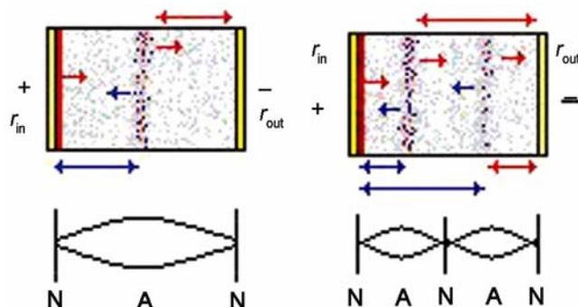
Figure 5. Standing wave(s) of pressure in an ozonizer.
