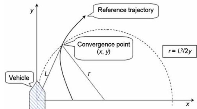
**Figure 6.** Pure pursuit algorithm determines the radius of curvature  $r$  with which the vehicle should move to converge to the reference trajectory at a distance  $L$  (look-ahead distance).
