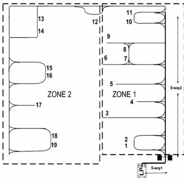
**Figure 8.** Shared AGV tracks, s-way 1 and s-way 2, shown with dark lines.
