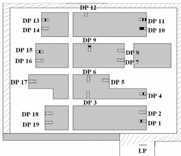
**Figure 1.** Layout of a machine shop floor. There is a single loading point (LP) and 19 delivery points (DP). The grey areas are to be avoided by the automated guided vehicle (AGV). The hatched area indicates the main corridor available for AGV movement.
