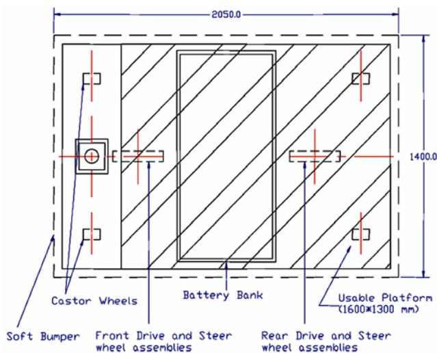
Figure 3. AGV wheel configuration.
