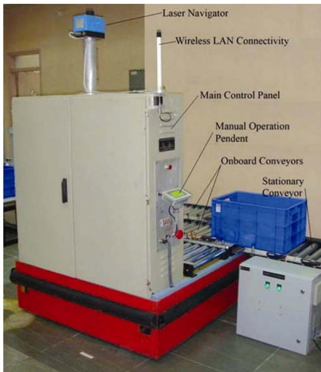
Figure 4. The automated guided vehicle.
