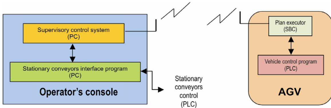
Figure 2. Intelligent material distribution system control architecture.
