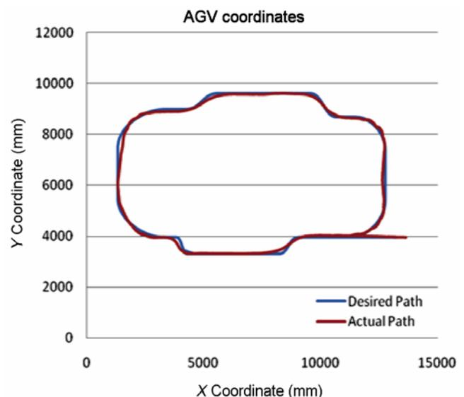
**Figure 7.** Path actually followed by AGV against the reference path.
