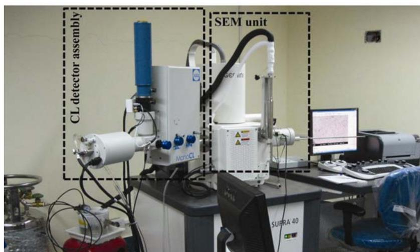
**Figure 2.** Photograph of the CL-SEM system installed at the Saha Institute of Nuclear Physics, Kolkata.
