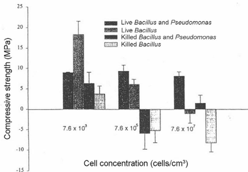
Figure 1. Increase in strength of cement with respect to bacterial concentration<sup>14</sup>.
