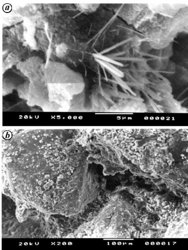
Figure 4. Comparison of SEM photomicrographs of mortar<sup>21</sup>. (a) With microorganism and (b) without microorganism.
