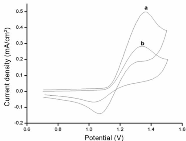
**Figure 4.** Cyclic voltammogram of LB medium containing  $30\text{ mg/l}$  Cr(VI) (a) before and (b) after *P. aeruginosa* treatment. Rest time,  $5\text{ s}$  and scan rate,  $10\text{ mV/s}$ .
