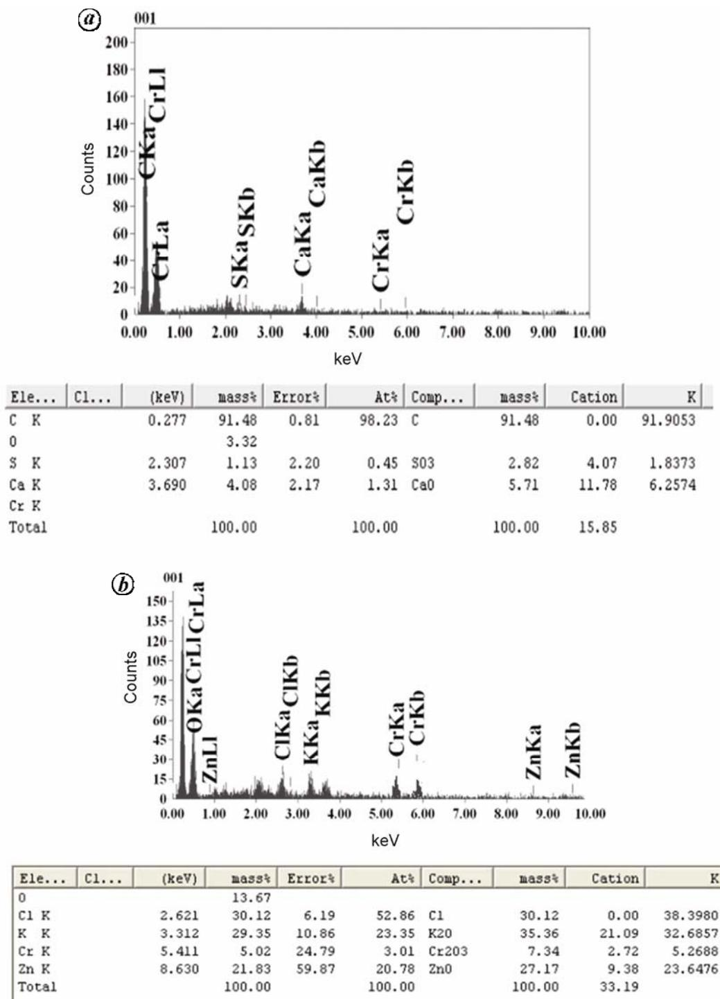
Figure 7. EDX of *P. aeruginosa*. (a) Control and (b) Cr(VI)-treated.
