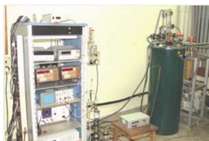
**Figure 8.** The high-field SQUID magnetometer set-up.
