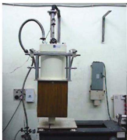
**Figure 14.** The SQUID-based NDE setup.
