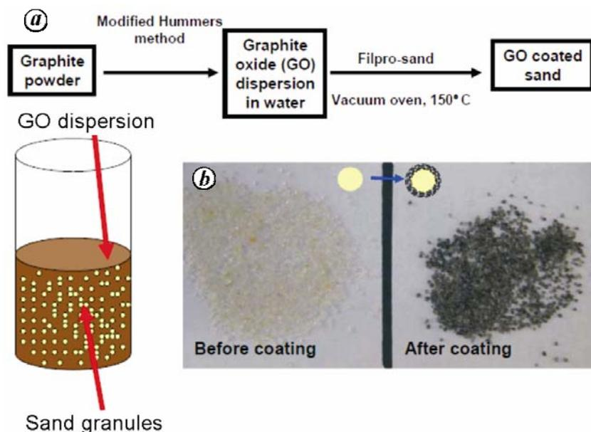
**Figure 3.** **a**, Flow chart and schematic illustration for the preparation of  $\text{GO}_{\text{SAND}}$ . **b**, Photographic images of sand and  $\text{GO}_{\text{SAND}}$  product. (Inset) Idealized schematic of conversion of regular sand to  $\text{GO}_{\text{SAND}}$ . Reprinted with ACS permission from Gao *et al.*<sup>16</sup>. Copyright (2011) from American Chemical Society.
