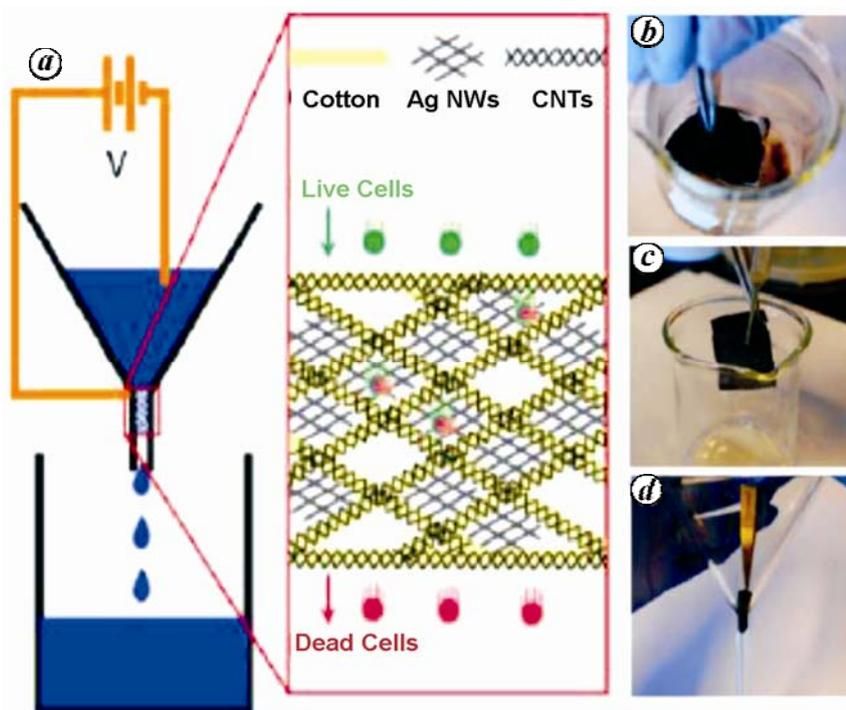
**Figure 1.** Schematic fabrication and structure of cotton, silver nanowire (AgNW)/carbon nanotube (CNT) device. **a**, Schematic active membrane device proposed. **b**, Treatment of cotton with CNTs. **c**, Treatment of device with AgNWs. **d**, Integration of treated cotton into funnel. Reprinted with ACS permission from Schoen *et al.*<sup>15</sup>. Copyright (2011) from American Chemical Society.
