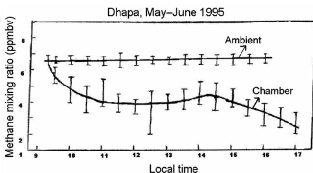
**Figure 1.** Methane emission values expressed in terms of mixing ratio at different times of the day during a dry season. Corresponding ambient values are also shown.
