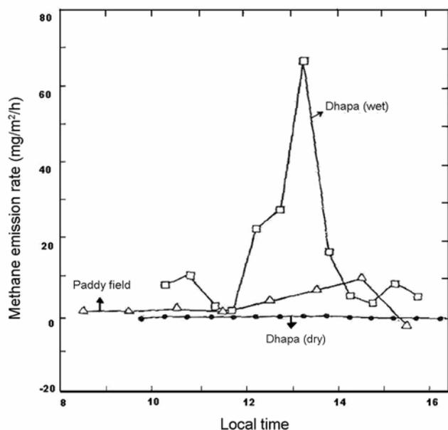
**Figure 3.** Typical methane emission rates for Dhapa for both dry and wet seasons and for the paddy field.
