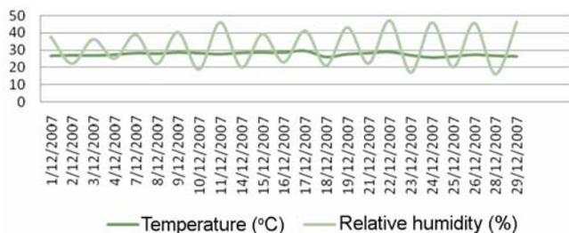
**Figure 1.** Relative humidity and temperature outside cave no. 2 at Ajanta.
