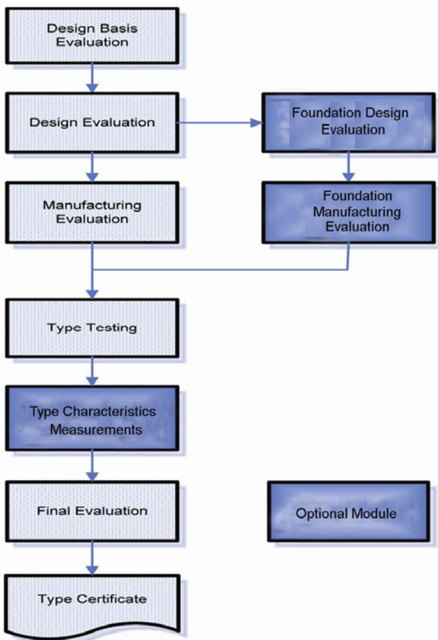
Figure 10. Type certification procedure according to IEC 61400-22.
