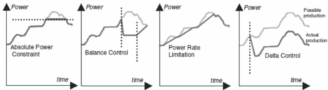
Figure 6. Potential wind farm control mechanisms to regulate grid loading<sup>15</sup>.
