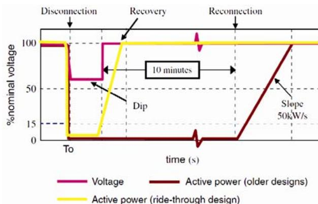
**Figure 5.** Active power ride-through for wind turbine operation during short grid intermissions<sup>14</sup>.
