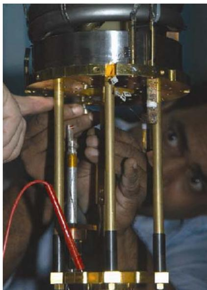
**Figure 10.** Platinum NMR thermometer mounted on a silver holder.
