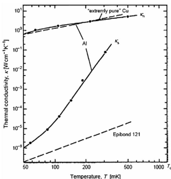
**Figure 7.** Thermal conductivity of superconducting and normal aluminium along with that of copper and ‘epibond’.
