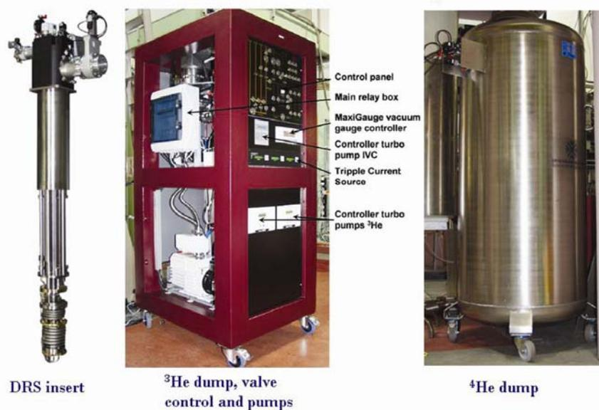
**Figure 2.** The DRS1000 dilution refrigerator. (Left) Dilution insert. (Middle) Pump housing, valve system and  $^3\text{He}$  dump. (Right)  $^4\text{He}$  dump.
