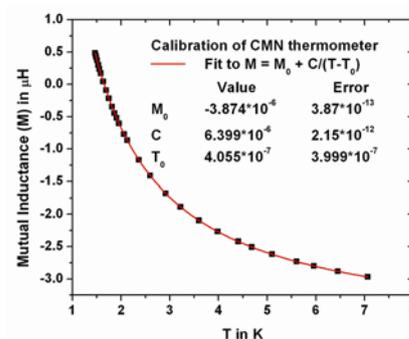
**Figure 9.** Initial calibration of the cerium magnesium nitrate (CMN) susceptibility thermometer against the SPEER resistance thermometer according to Curie–Weiss law.  $T_0$  is very small and is therefore neglected.
