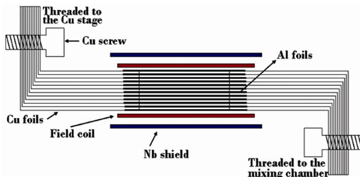
**Figure 8.** Schematic of the superconducting heat switch.
