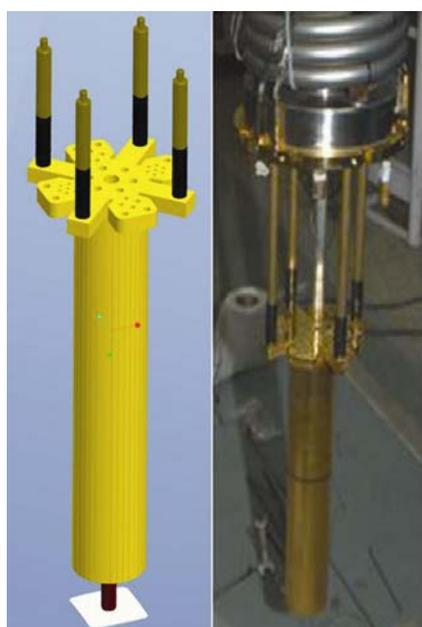
**Figure 5.** (Left) Diagrammatic sketch of the copper nuclear stage. (Right) Actual copper stage in our laboratory.
