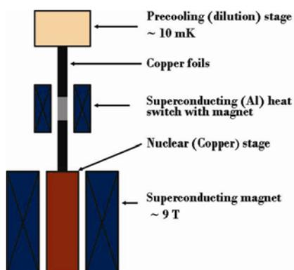
Figure 1. Schematic of an adiabatic nuclear demagnetization set-up.
