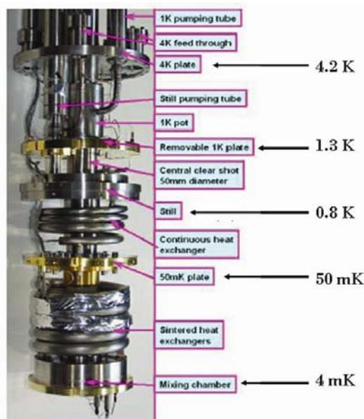
**Figure 3.** The dilution refrigerator stages showing a gradual lowering of temperature from the top 4 K plate.
