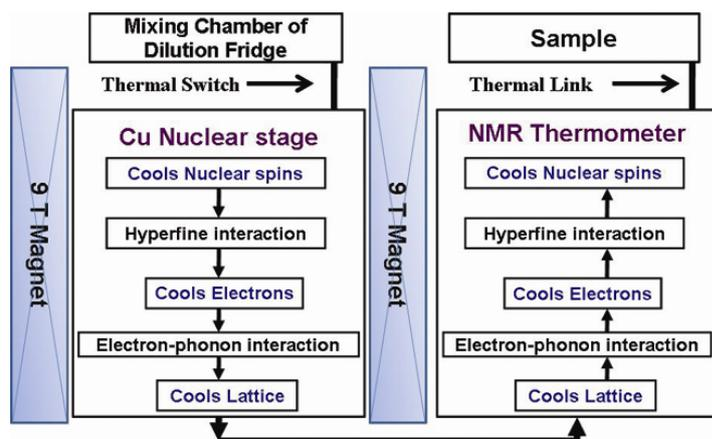
**Figure 13.** Various cooling mechanisms at play in nuclear cooling and NMR thermometry.
