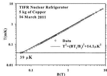
**Figure 15.** The  $B$  versus  $T$  curve during demagnetization. The continuous line is a fit to eq. (1) in the text.
