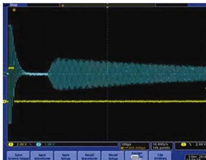
**Figure 12.** Free induction decay (FID) curve at 39  $\mu\text{K}$ . Notice the excitation pulses before the FID curve.
