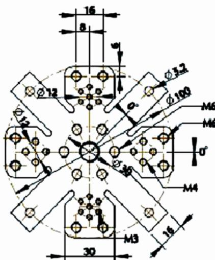
**Figure 6.** Threaded holes on the copper stage for mounting experiments.
