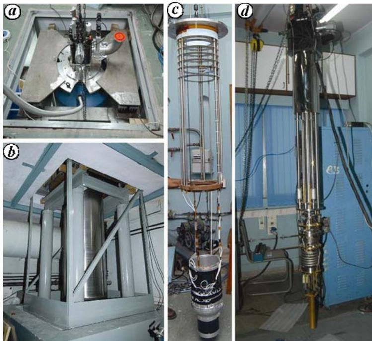
**Figure 14.** *a*, Cryostat mounted on active vibration isolation pads. *b*, Cryostat hanging into the basement on pillars resting on a sand-bed. *c*, Magnet insert. *d*, Dilution insert with the copper stage.
