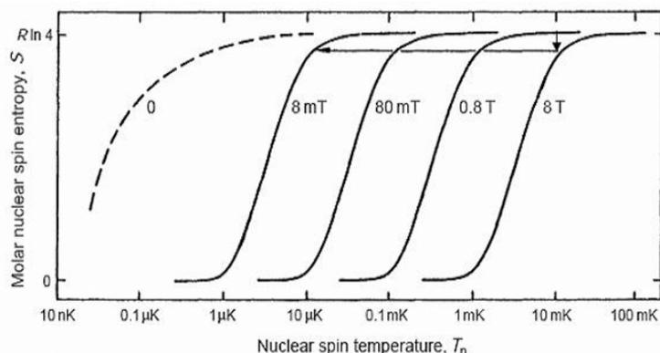
**Figure 4.** Entropy versus temperature curves of the Copper nuclear spin system at different fields<sup>2</sup>.
