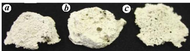
**Figure 1.** Silver monoliths after calcination. *a*, Ag sponge after calcination of Ag/Triton X-305 xerogel. *b*, Ag monolith after calcination of Ag/Triton X-305/dextran xerogel. *c*, Ag framework after calcination of Ag/Triton X-305/TMB xerogel.
