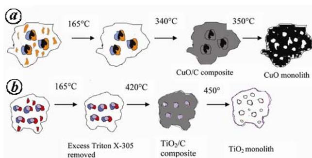
**Figure 6.** Morphological transformations of CuO and TiO<sub>2</sub> monoliths. *a*, CuO/Triton X-305/dextran. *b*, TiO<sub>2</sub>/Triton X-305/dextran. Black colour, CuO; red, Triton X-305; blue, dextran; grey, carbon and violet/white, TiO<sub>2</sub>.
