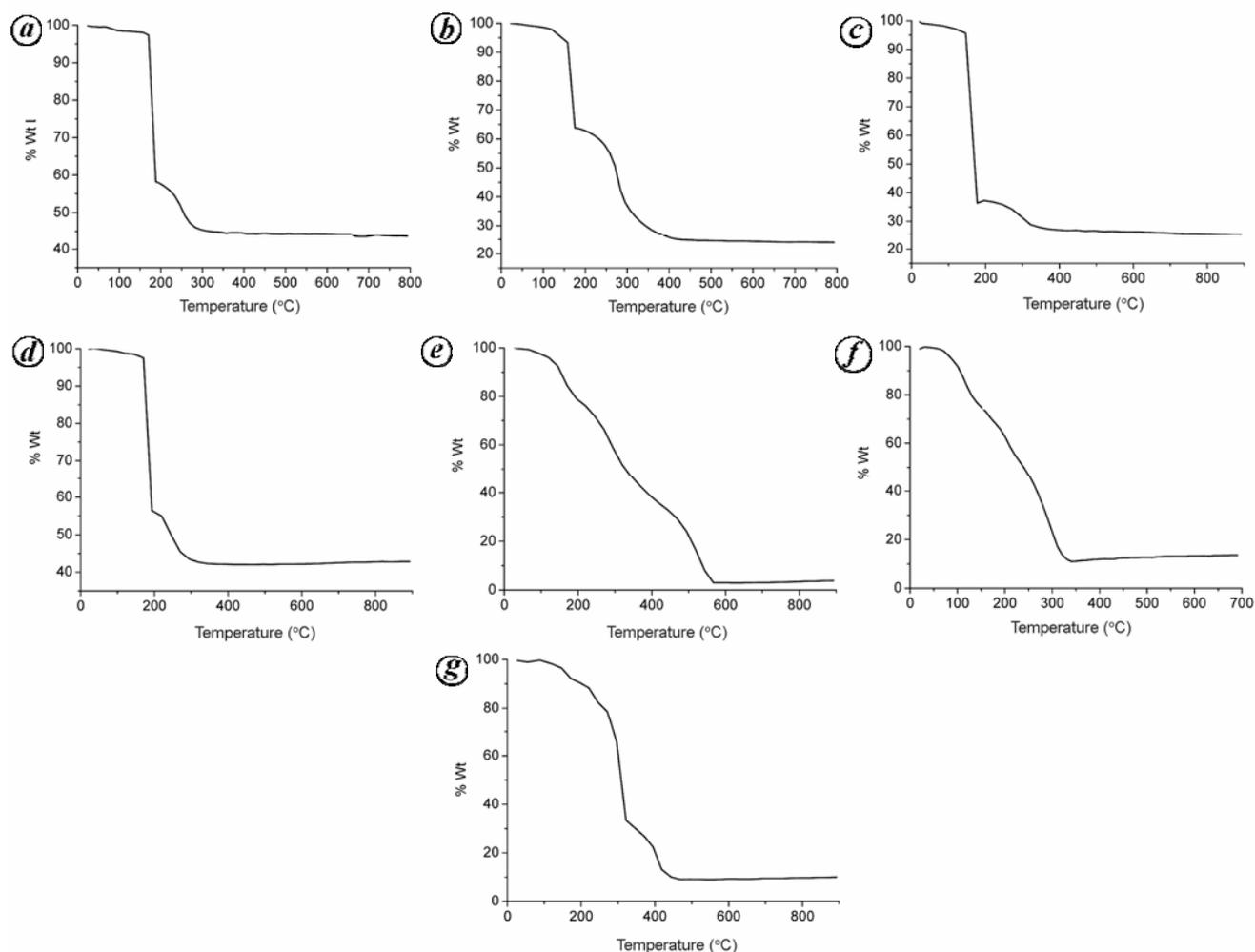
**Figure 5.** Thermogravimetric analysis graphs for various xerogels: *a*, Ag/Triton X-305; *b*, Ag/Triton X-305/dextran; *c*, Ag/Triton X-305/ludox; *d*, Ag/Triton X-305/TMB; *e*, Au/Triton X-305/dextran; *f*, Copper nitrate/Triton X-305/dextran, and *g*, TiO<sub>2</sub>/Triton X-305/dextran.
