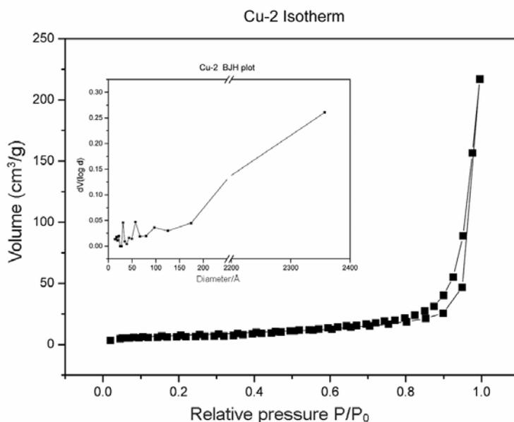
**Figure 7.** The Brunauer, Emmitt and Teller  $N_2$  adsorption isotherm plots for CuO monolith prepared by the calcination of copper nitrate/Triton X-305/dextran xerogel. (Inset) Micropore size distribution.
