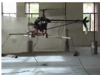
**Figure 3.** Attitude control of a mini helicopter under tethered hover flight.
