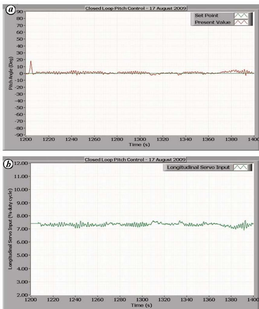
Figure 2. *a*, Pitch angle response of the mini helicopter with closed loop control. *b*, Control input during pitch stabilization of the mini helicopter.
