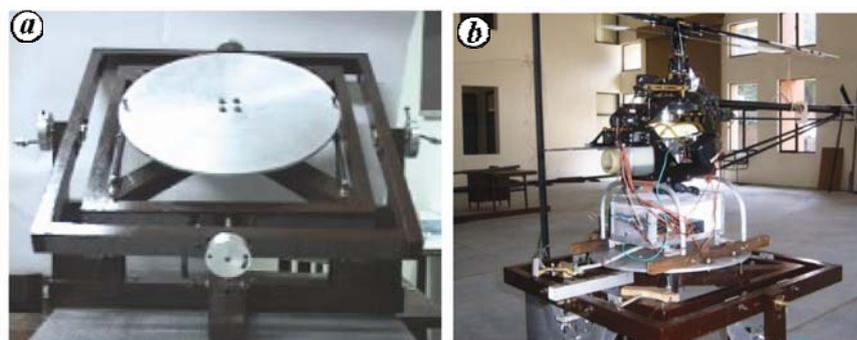
Figure 1. *a*, Three-axis test rig. *b*, Model helicopter mounted on the three-axis test rig.
