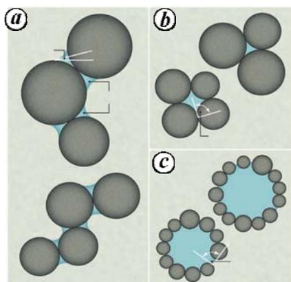
**Figure 1.** Schematic representation showing the stabilization of suspensions and emulsions with a third added phase. **a**, Pendular state; **b**, Capillary state; **c**, Pickering emulsion. (From Butt<sup>5</sup>, reprinted with permission from AAAS.)
