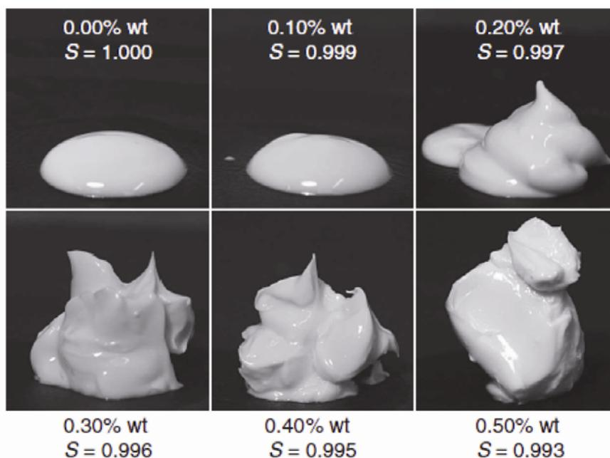
**Figure 2.** Photograph illustrating the transition from a weakly elastic behaviour to highly elastic gel-like behaviour by the addition of small amounts of water to a suspension of hydrophobically modified calcium carbonate in DINP. (From Koos and Willenbacher<sup>4</sup>, reprinted with permission from AAAS.)
