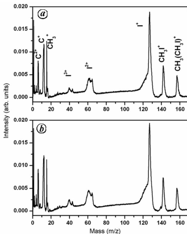
**Figure 13.** Time-of-flight mass spectra of  $\text{CH}_3\text{I}$  clusters at 532 nm under (a) parallel ( $0^\circ$ ) and (b) perpendicular ( $90^\circ$ ) polarization.
