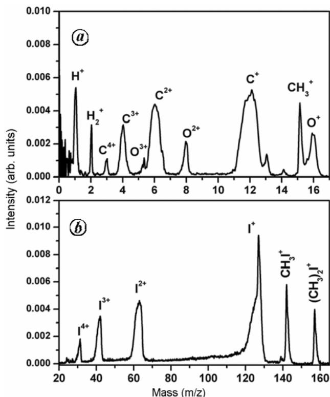
**Figure 14a, b.** Time-of-flight mass spectra of  $\text{CH}_3\text{I-H}_2\text{O}$  mixed clusters when subjected to 563 nm laser pulse at an intensity of  $\sim 10^9 \text{ W/cm}^2$ .
