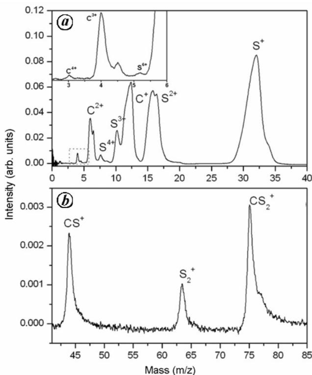
**Figure 5 a, b.** Time-of-flight mass spectra of carbon disulphide clusters subjected to 532 nm laser pulse of intensity  $\sim 10^9 \text{ W/cm}^2$ .
