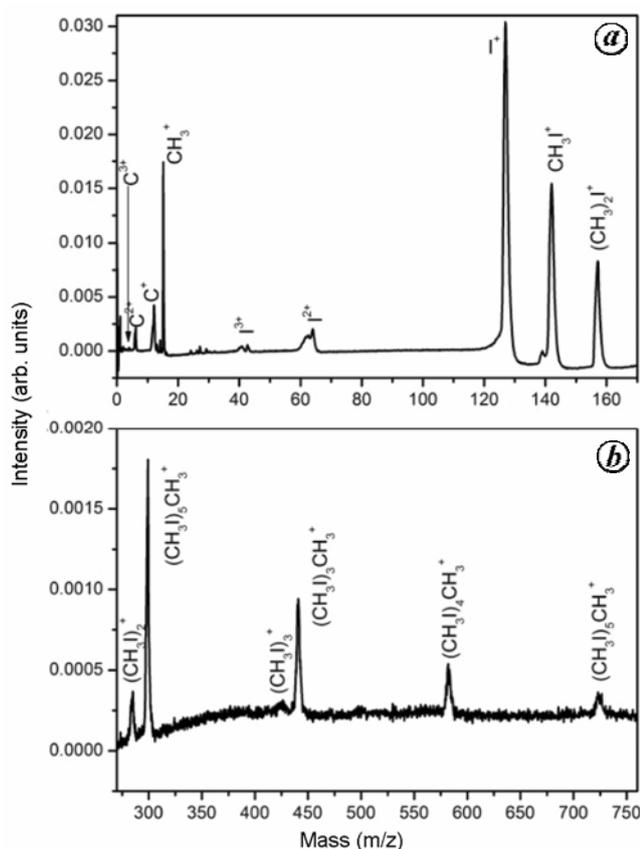
**Figure 4 a, b.** Time-of-flight mass spectra of methyl iodide clusters subjected to 532 nm laser pulse of intensity  $\sim 10^9$  W/cm<sup>2</sup>.
