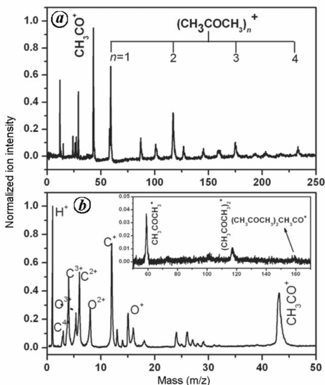
**Figure 8.** Time-of-flight mass spectra recorded for acetone clusters at 532 nm using (a) 0.5 mm and (b) 0.8 mm diameter nozzle.
