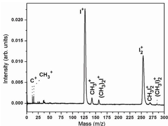
**Figure 2.** Time-of-flight mass spectra of methyl iodide clusters upon multiphoton excitation at 266 nm.
