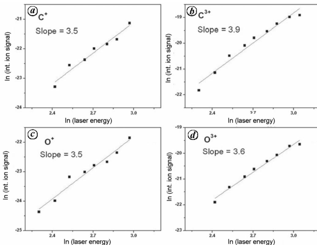
**Figure 11.** In–ln plots for multiply charged ions generated upon interaction of 532 nm laser pulse with acetone clusters.
