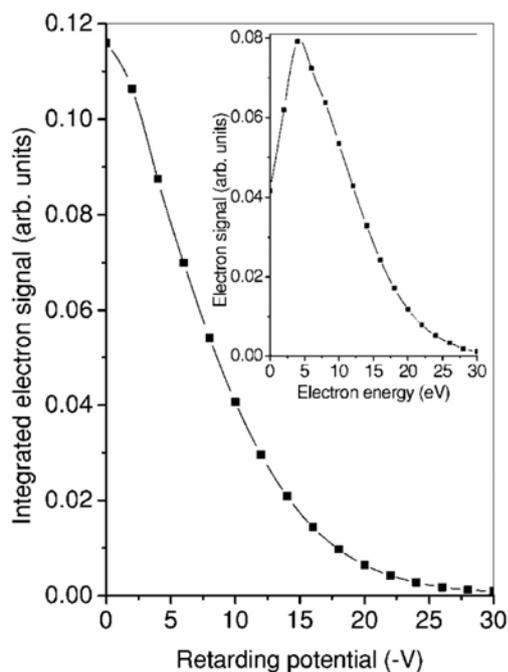
**Figure 12.** Integrated electron signal as a function of retardation potential for methyl iodide clusters at 532 nm. (Inset) Area-normalized electron energy distribution generated from the integrated data.
