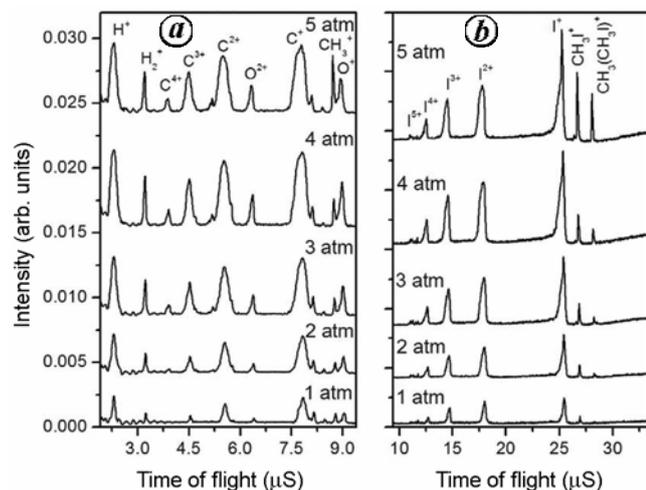
**Figure 7.** Variation in ion signal of multiply charged ions as a function of helium back-up pressure for methyl iodide clusters: *a*,  $C^{p+}$  ( $p \leq 4$ ) and *b*,  $I^{q+}$  ( $q \leq 5$ ).
