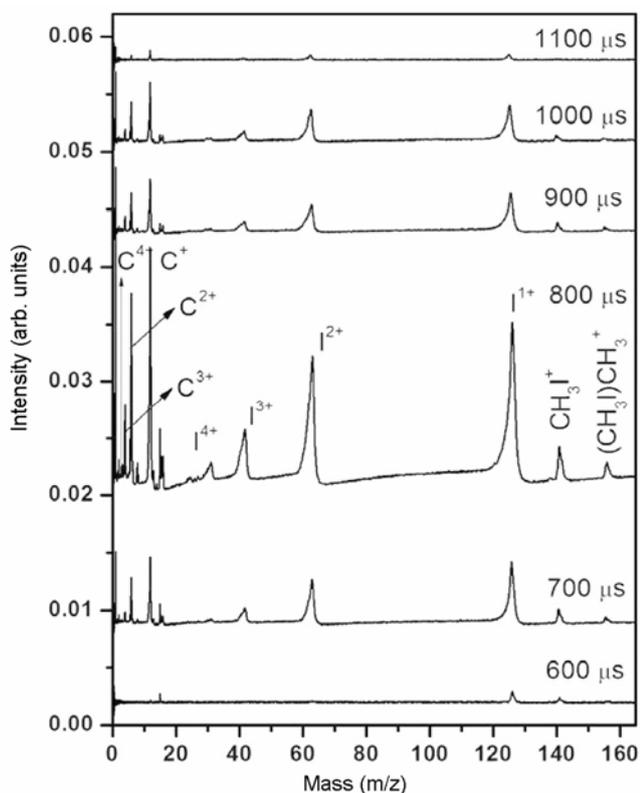
**Figure 6.** Variation in ion signal of multiply charged ions as a function of delay between pulsed valve and laser firing for clusters of methyl iodide at 563 nm.
