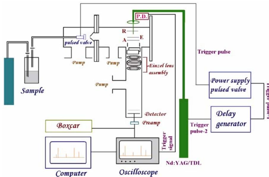
**Figure 3.** Schematic layout of cluster set-up designed and fabricated at the Chemistry Division, Bhabha Atomic Research Centre, Trombay.
