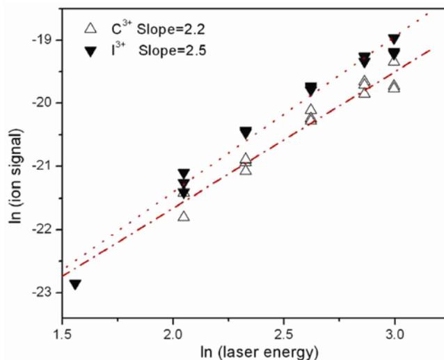
**Figure 10.** In–ln plot of laser energy versus signal intensity of multiply charged fragment ions ( $\text{C}^{3+}$  and  $\text{I}^{3+}$ ) that are produced upon interaction of  $\text{CH}_3\text{I}$  clusters with 532 nm laser pulse of  $\sim 10^9$   $\text{W}/\text{cm}^2$  intensity.
