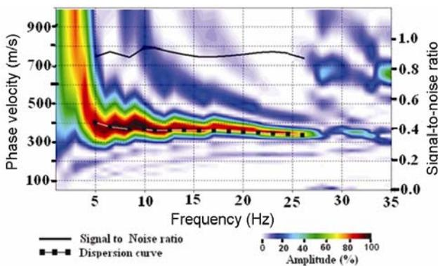
Figure 3. Typical dispersion curve.
