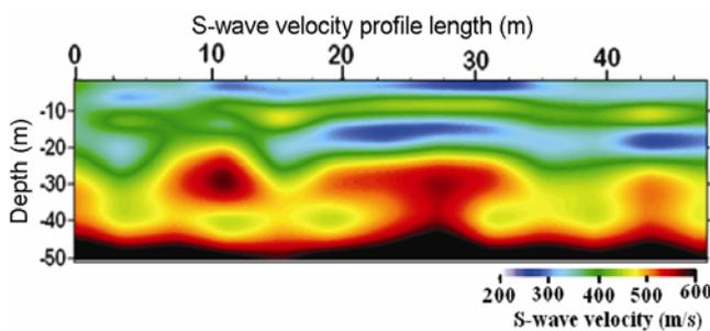
Figure 4. Typical 2D velocity profile.
