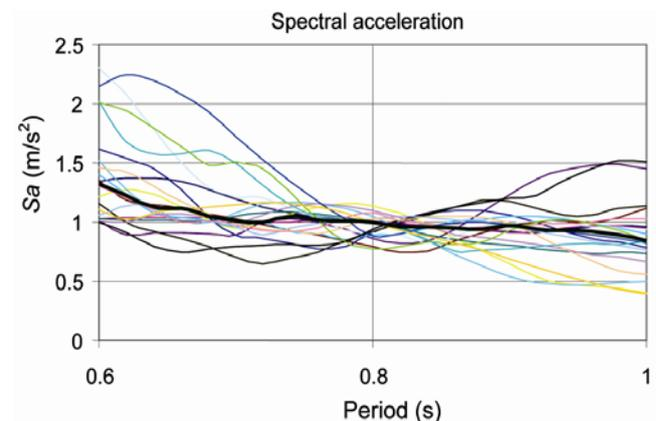
**Figure 4.** Variation of  $Sa$  when scaled to  $Sa, \text{median}, 0.6 \text{ s} \leq T_n \leq 1.0 \text{ s}$  for individual ground motions (thick line shows median values).
