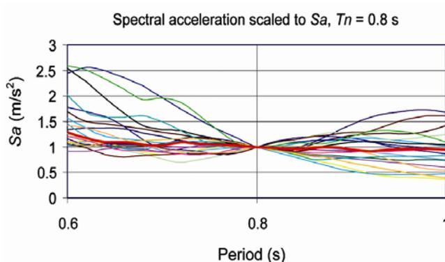
**Figure 3.** Variation of  $Sa$  when scaled to  $Sa, T_n = 0.8 \text{ s}$  for individual ground motions (thick line shows median values).
