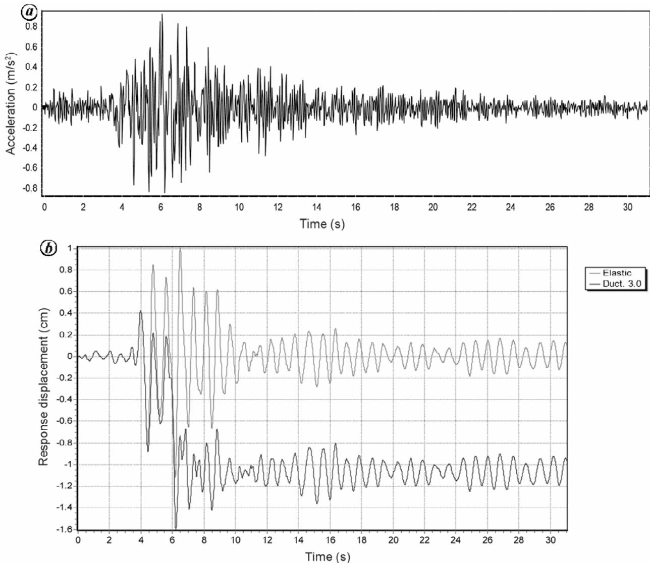
Figure 1. LMLR1 time history (a) and inelastic displacement response (b).
