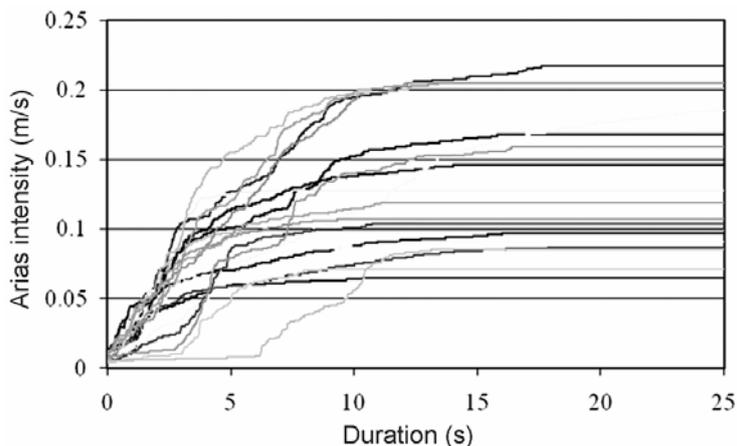
Figure 5. Build-up of Arias intensity for individual ground motions.
