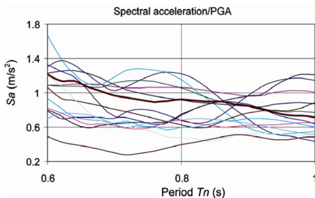
**Figure 2.** Variation of spectral acceleration ( $Sa$ ) when scaled to unit peak ground acceleration (PGA) for individual ground motions (thick line shows median values).
