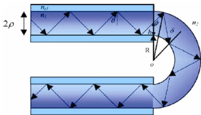
**Figure 1.** Geometry of a U-shaped sensing region and representation of a meridional ray in it.
