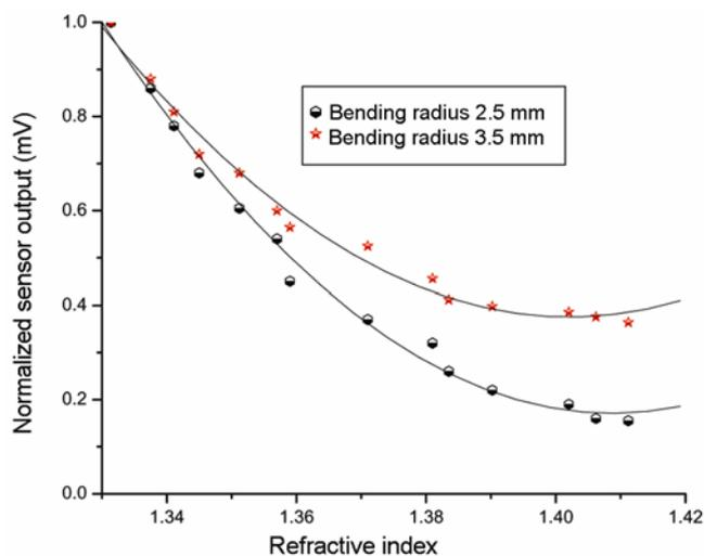
Figure 4. Normalized sensor response for different bending radii.
