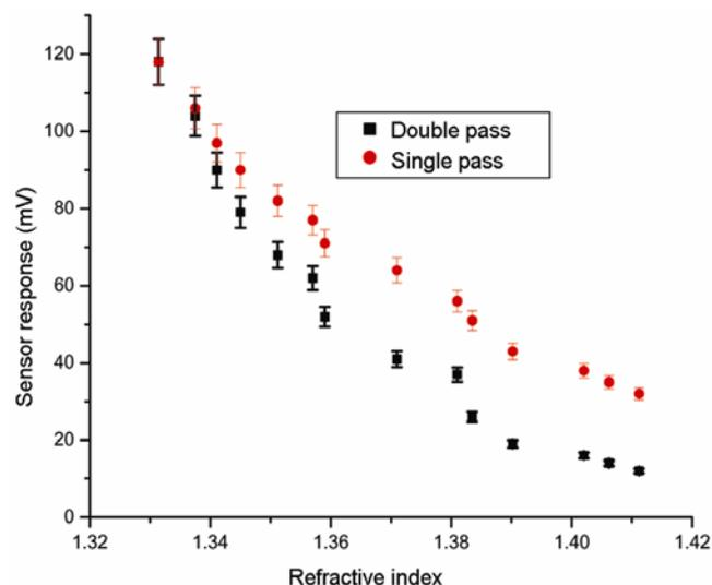
**Figure 3.** Sensor response for single pass and double pass evanescent field absorption.
