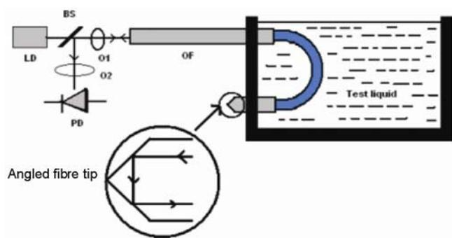
**Figure 2.** The experimental arrangement for the present fibre optic sensor. LD, Laser diode; BS, Beam splitter; O1, Objective; O2, Objective; OF, Optical fibre, and PD, Photodiode.
