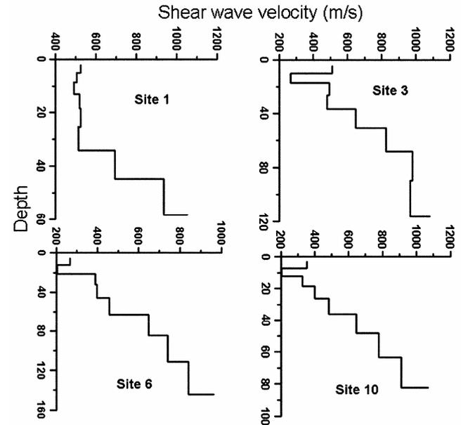
Figure 5. One-dimensional shear wave velocity with depth at different sites of the Dehradun fan.
