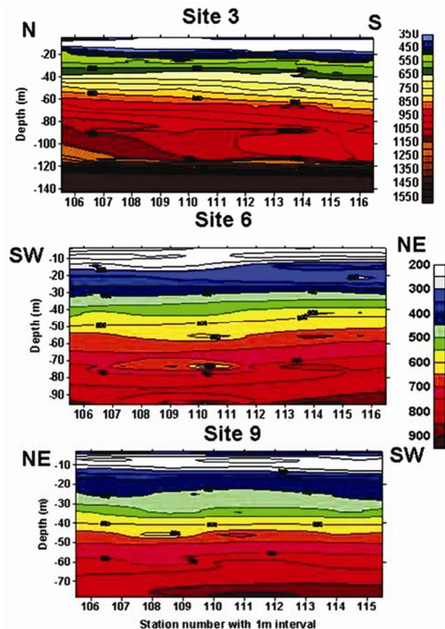
Figure 4. Two-dimensional velocity model of different sites from north to south depicting shear wave velocity.
