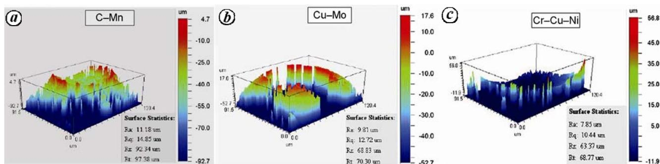
**Figure 2.** Typical results from profilometer analysis at the starting portion of the crevice (location 1). *a*, C–Mn steel sample; *b*, Cu–Mo and *c*, Cr–Cu–Ni rail steel sample on immersion in 3.5% NaCl + 3.5% FeCl<sub>3</sub> solution after 30 days.
