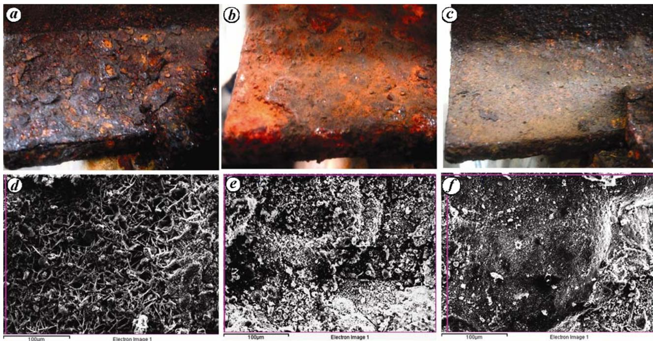
**Figure 3.** Macro images of foot portion of rail steel: *a*, C–Mn; *b*, Cu–Mo and *c*, Cr–Cu–Ni and corresponding microscopic features (observed by SEM) of outer rust on the rail steels. *d–f*, After six months of salt fog exposure showing the lower rusting and compact rust formation in the case of Cr–Cu–Ni rail steel.
