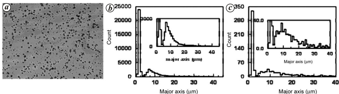
**Figure 1.** *a*, Photomicrograph of CR-39 detector 10-5 obtained at 200 $\times$  magnification. The detector had been etched in 6.5 N NaOH at 65 $^{\circ}$ C for 7 h. *b*, *c*, Scanned results obtained for CR-39 detector 10-5: *b*, for the front surface (34,254 tracks) and *c*, for the back surface (750 tracks).
