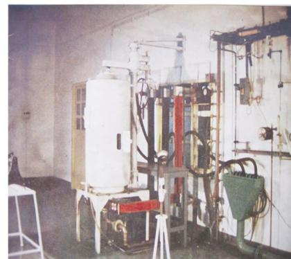
**Figure 5.** Commercial-scale pilot polysilicon reactor with quartz bell jar and shield.
