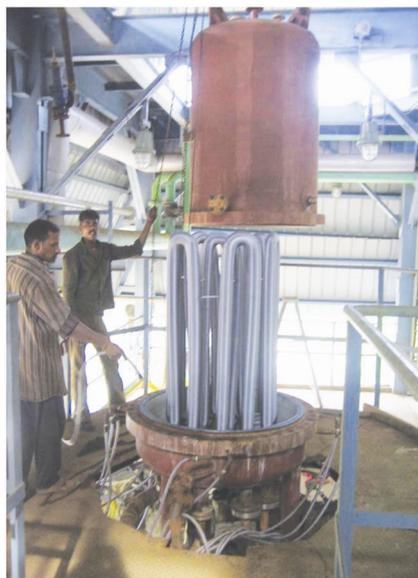
**Figure 8.** Polysilicon reactor being opened after completion of a deposition run.
