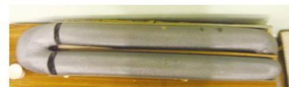
**Figure 6.** Fully grown polysilicon hairpin.
