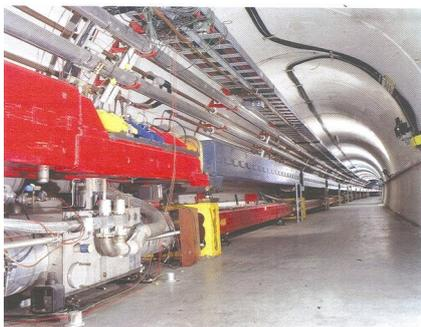
The conventional-magnet Main Ring synchrotron (top) and the Tevatron (bottom) within their 6.3-km enclosure. During the initial stages of Tevatron operation, the Main Ring served as an injector into the Tevatron and as the source of protons for antiproton production. Later in the Tevatron era, this role was assumed by the Main Injector, and the Main Ring was decommissioned.
