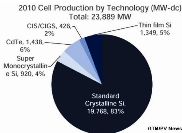
**Figure 1.** Break-up of global photovoltaic technologies.
