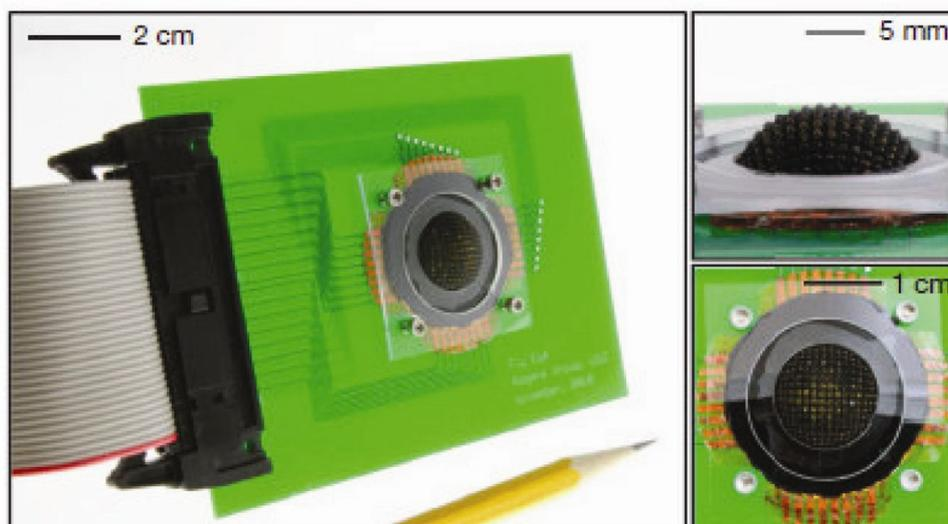
**Figure 2.** Photograph of the completed bio-inspired digital camera mounted on a printed circuit board. (Reprinted with permission from Song *et al.*<sup>1</sup>, Copyright (2013) Nature publishing group.)
