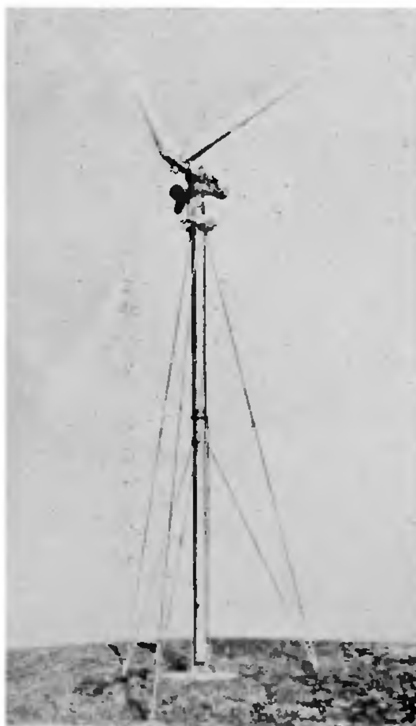
FIG. 1. 6 kW Allgaier wind electric generator with three blades, each 5 metres long.
